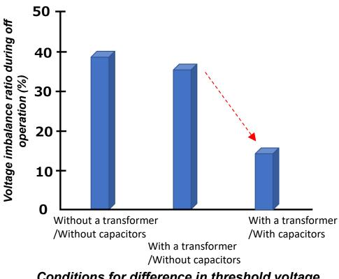
Conditions for difference in threshold voltage (No difference in gate signal)
