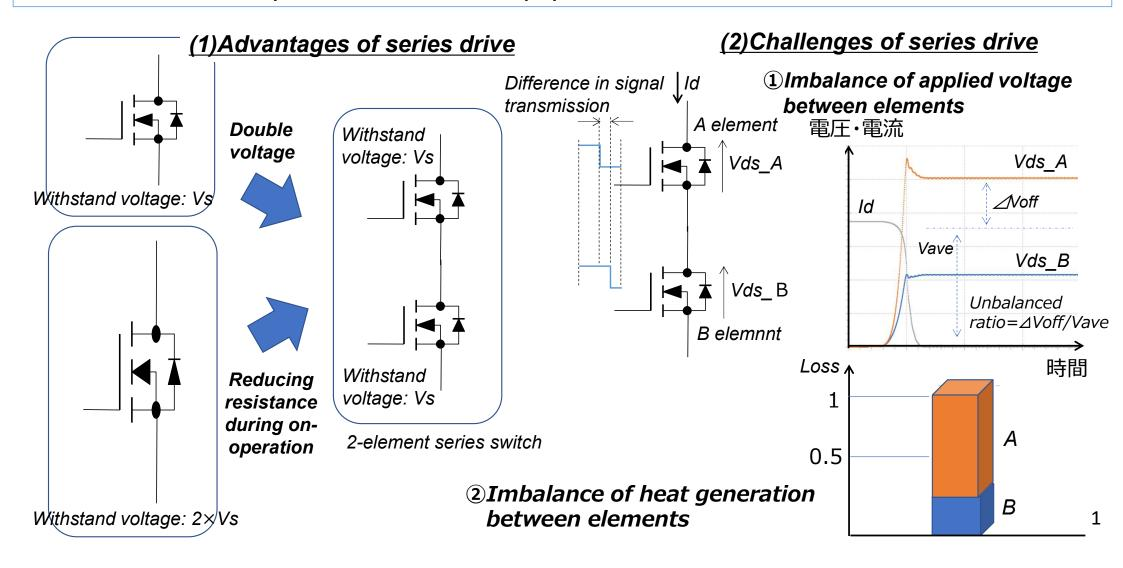
1. When the magnetic coupling method (1) is used to drive SiC power semiconductors in series, the effects of gate signal and gate voltage deviation are verified using a circuit simulator.
